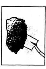
APPLY: Shovel or pour UPM® mix into the hole. Level out 25% higher than the existing pavement to allow for compaction. If patch is deeper than 4", apply and compact in separate 2" layers.
